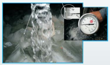
1. At the RMC plant, the concrete temperature was reduced significantly by using chilled water and ice cubes.
